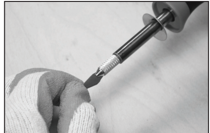
Wear gloves when attaching the hot knife tip
